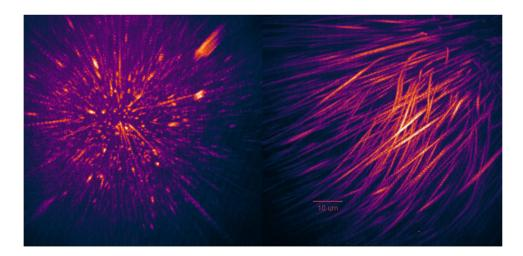
**Painting Fireworks:** Thin films of paint dry fast, leading to fluid instabilities which result in defects in the final coating. Marangoni stress creates beautiful recirculation patterns, leaving a mottled appearance in the dried film. Multiple Particle Tracking (MPT) microrheology of drying paints "explodes like fireworks", exposing their material properties.
