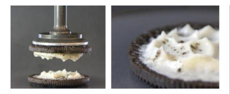
**FIGURE 3**. (Left) Perfectly separated Oreo using the HCP at 65°C. (Right) Close-up image of the lower wafer, with a satisfying amount of creme.
