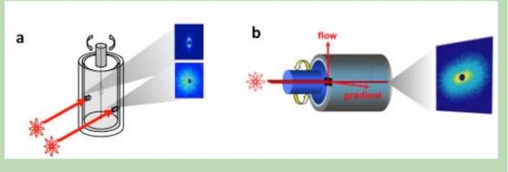
Figure 3. a) Geometry for *tOr-SANS* experiments in the 1,3 and 2,3 planes of flow and b) new geometry that directly probes the shear plane (1,2 plane of flow) (adapted from Helgeson et al. "Neutron transmission measurements of concentration profiles in non-homogeneous shear flows," 2010 Annual Report, NIST Center for Neutron Research, Gaithersburg, MD. p. 38-39, 2010).
