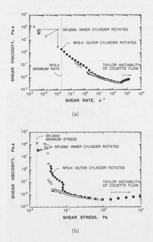
Figure 3 Shear viscosity of the supernatant liquid in Orbitz<sup>TM</sup> versus (a) shear rate, and the same data replotted versus (b) shear stress. Couette fixtures were used in both the rheometers. When the inner cylinder rotates and the shear rates exceed 500 s<sup>-1</sup>, the critical Taylor number for the onset of vortices in the annular gap is exceeded; the ensuing secondary flow may raise the apparent viscosity.
