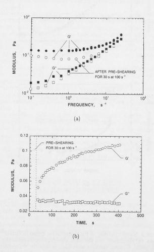
Figure 2 Elastic and viscous moduli of the supernatant liquid. (a) Versus frequency, with and without pre-shearing. (b) Versus time, after pre-shearing. The frequency was  $1 \text{ s}^{-1}$ , and the strain imposed was 10%.
