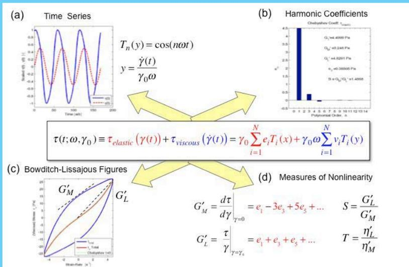
Figure 5. Various methods for plotting LAOS rheometry data.
