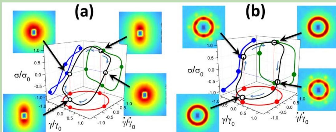
Figure 4. Stress response and SANS profiles during LAOS of (a) a 6 wt% aqueous solution of CPCl/NaSal, with molar ratio [NaSal]/[CPCl]=0.5 at 25 °C ( $\omega = 0.56$  rad/s and  $\gamma_0 = 10$ ) and (b) a 24 wt% Pluronic F127/EAN solution at 40 °C ( $\omega = 1$  rad/s and  $\gamma_0 = 100$ ). The arrows indicate the direction of oscillation.
