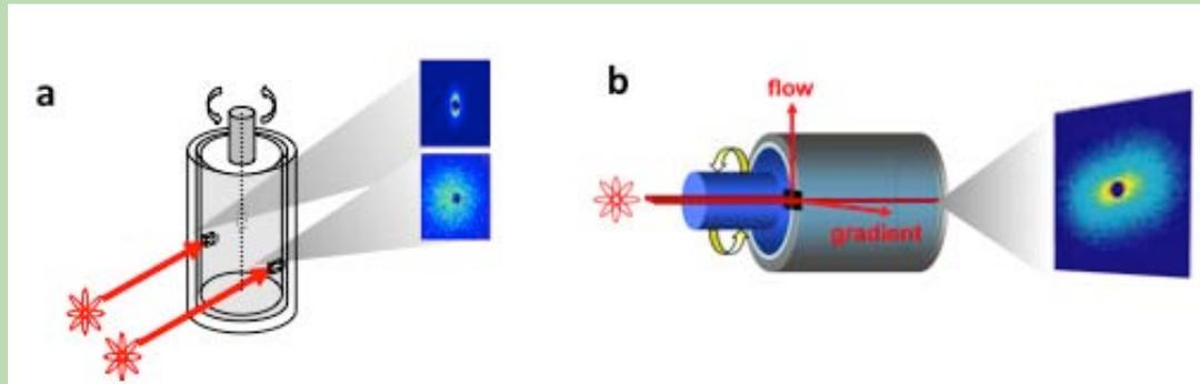
Figure 3. a) Geometry for *tOrSANS* experiments in the 1,3 and 2,3 planes of flow and b) new geometry that directly probes the shear plane (1,2 plane of flow) (adapted from Helgeson et al. "Neutron transmission measurements of concentration profiles in non-homogeneous shear flows," 2010 Annual Report, NIST Center for Neutron Research, Gaithersburg, MD. p. 38-39, 2010).
