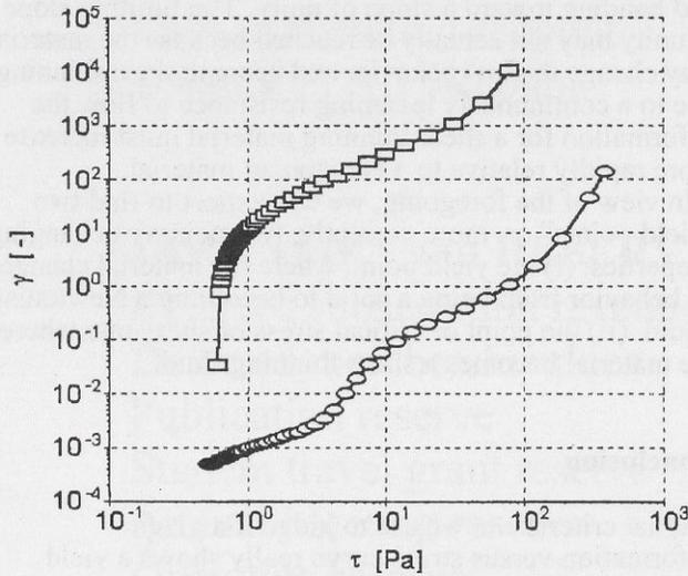
Figure 2 Practically observed deformation versus stress curves.
