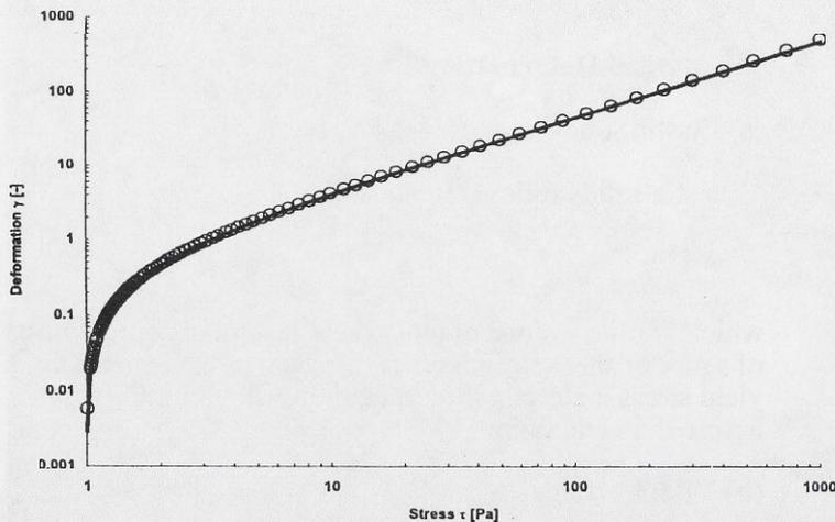
Figure 5 Measured and calculated deformation as a function of stress for a Newtonian oil of 100 Pa-s viscosity. The stress is increased logarithmically from 1 to 1000 Pa in 300 s.
