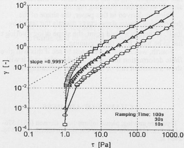
Figure 3 Influence of ramping time on the deformation versus stress behavior.
