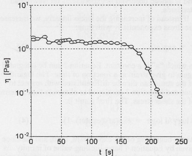
Figure 4 Viscosity versus time determined from data in yield point test.
