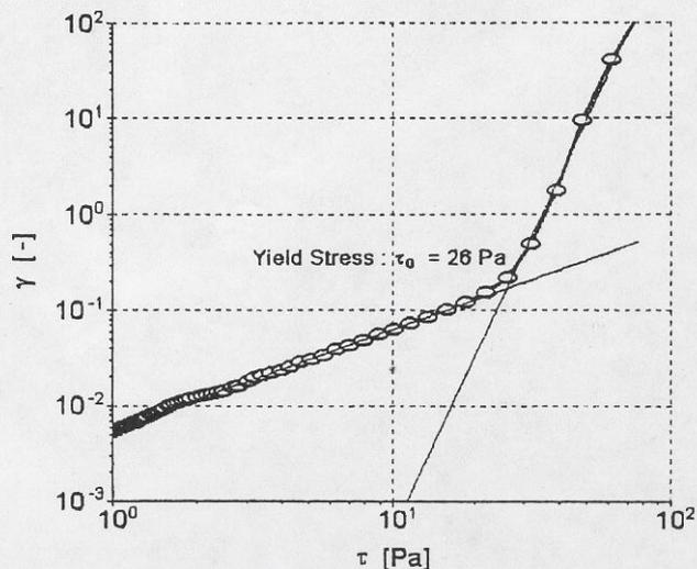
Figure 1 Typical deformation versus stress curve for a material with a yield point.
